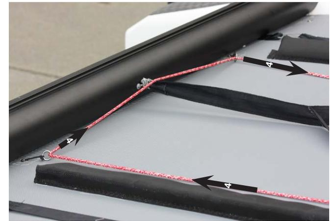
5. Feed the line through the 29mm block in front of the oval grommet and pull the line underneath the trampoline.
