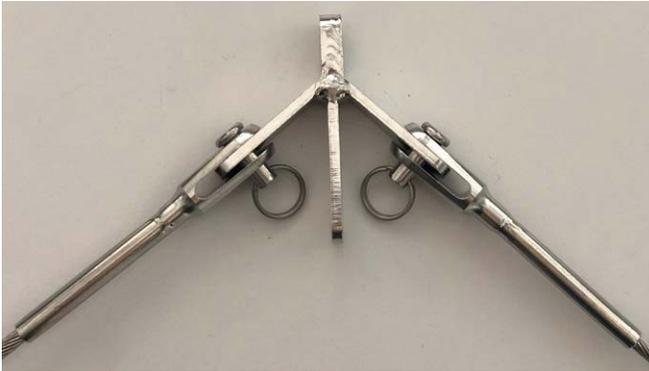
2. Install the ring 3x20 ss under the fork terminal on port side as shown in the picture.
