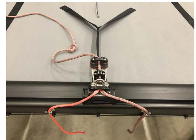
4. Knot the ends to the strapeyes. Make sure the traveler car is in the middle of the rear crossbar.
