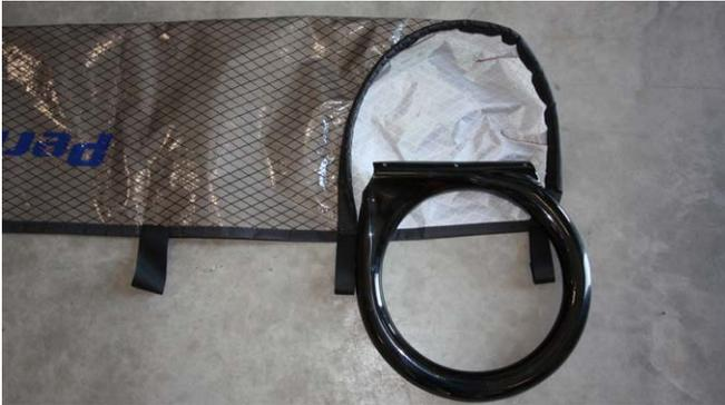
2. Slide the snufferbag into the slot of the snuffer ring.
