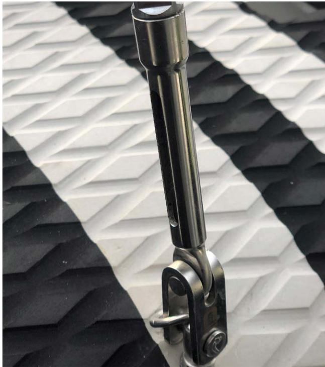
6. Install the adjustable trapeze with the shackle to the trapeze line. Check page 51 how to assemble the trapeze system.
