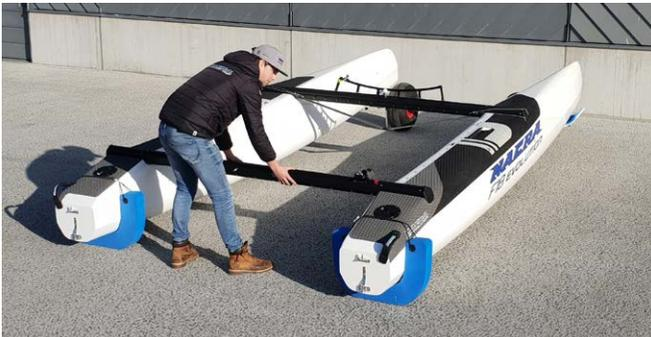
3. Grease the eight beambolts and make sure the fiberglass washer is at the bottom and the metal washer is on top. The washers for the front crossbar are already put in the slot on top of the front crossbar.
