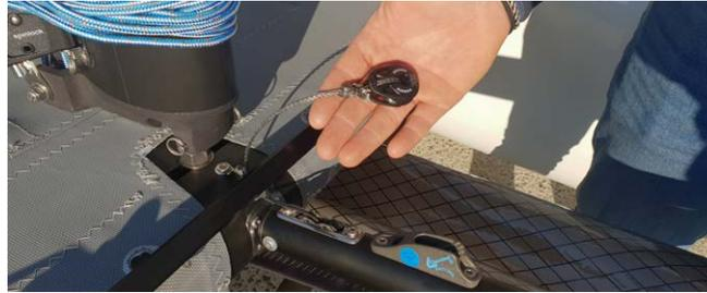
2. Feed the spinnaker halyard first through the 29mm T2 block and then through the 40mm block located on the mast.
