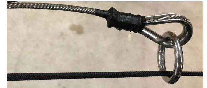
3. Knot one end with a bowline at the eyelet of the S-hook. The other end is attach with two bowlines unto the 1.6mm (short) jib halyard line. the loose end needs to be fed through the small hole in the S-hook and secured by a figure 8-Knot.
