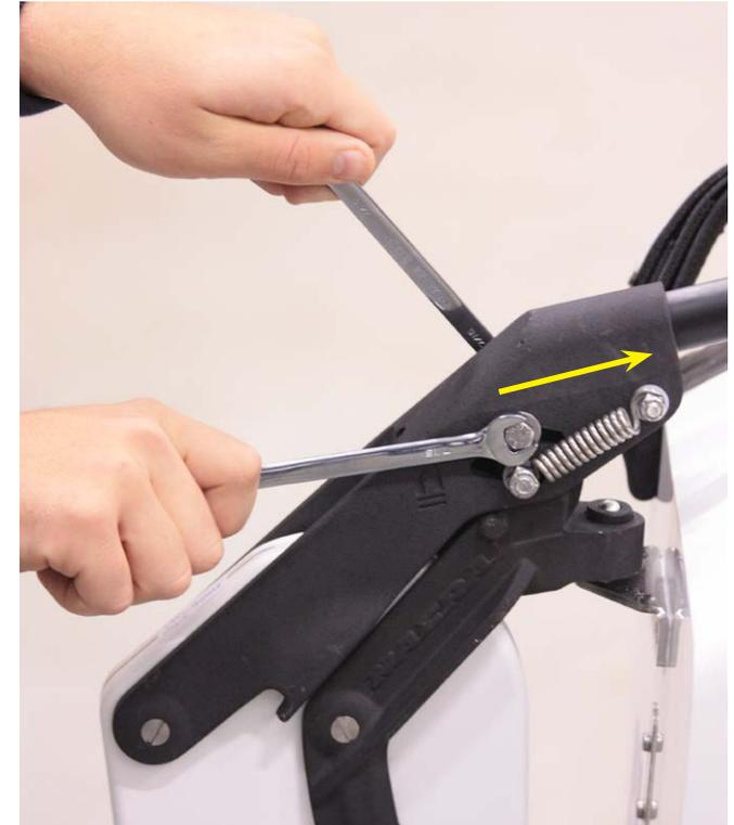
14. If you want to change the rudder rake, change the rubber for a smaller or bigger rubber.
