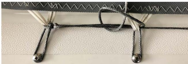
21. Continue until you reach the end of the line and install a security knot.
