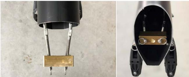
5. Grease the diamond adjuster bolt and adjust the washers and mastbase with the washer on top. Make sure the bolt is at least 5mm in the brass fitting.
