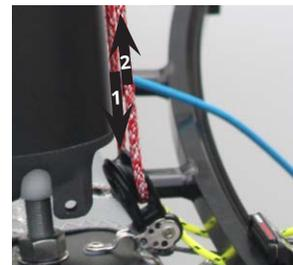
3. Feed the end of the spinnaker halyard (the one coming out of the cleat from the 40mm block) through the most front 29mm block on the trampoline.
