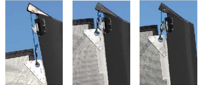
7. Slide the bottom part of the luff downwards into the masttrack.
