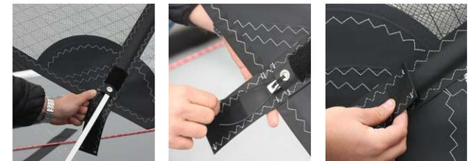
9. Insert the last DS batten in its pocket parallel to the mast. Tension it by using the velcro cover.
