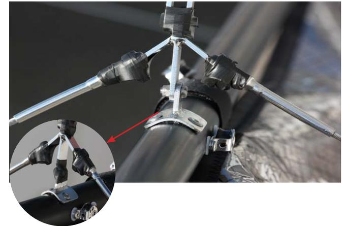
3. Push the bowsprit gently down in order to install the bowsprit bridle line on the bridle pin with the shackle narrow.
