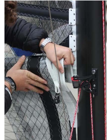
8. Insert the diagonal DS batten inside its pocket and tension it as described in **5.5 Battens**.
