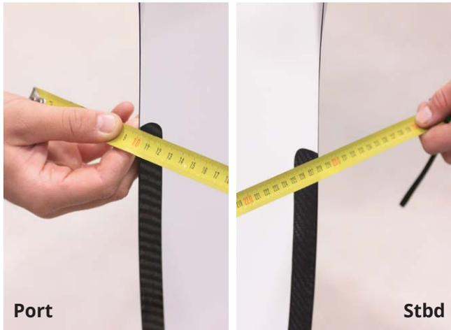
11. The rudders must face 2 mm inwards, this is adjustable by changing the rod length.
