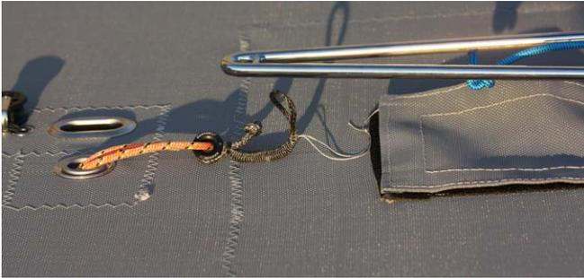
2. Feed the loop through to the mast rotator wishbone.
