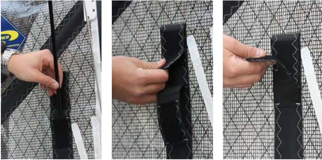
10. Install the two 29mm wire blocks on the loops at both sides of the mainsail.
