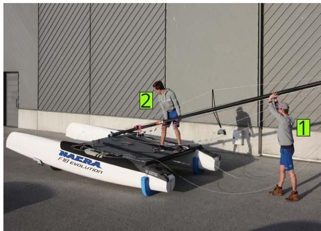
7. - **Person 1** Holds the mast up with one spreader arm facing downwards, so the mastbase doesn't hit the crossbar.
