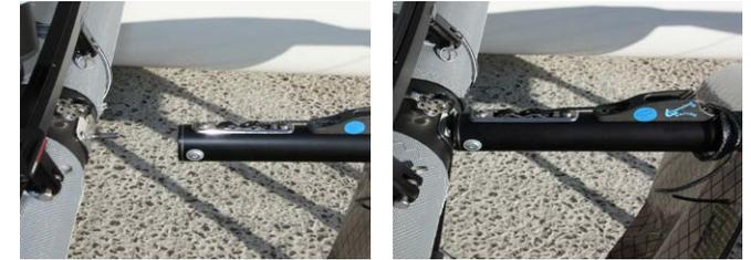
2. Install the bowsprit to the bridle connector, with the bolt and the nut.
