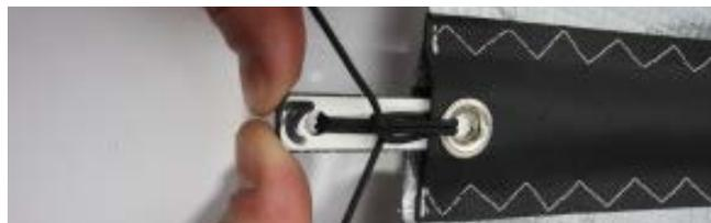
4. Finish tying with a square knot and tuck the loose ends in the batten pocket.
