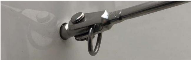
3. Place the mast with care on the trampoline with the masttrack down, support the back of the mast to prevent it from scratching!
