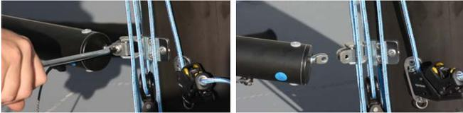
2. Attach the short line on the strapeye, mounted on the mast, with a bowline.
