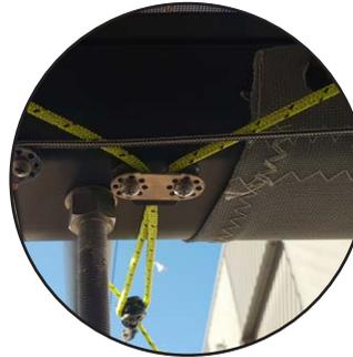
11. On port side, un-knot (from the small clamcleat) the rear pre-installed mouseline in the front crossbar, and attach it on the jibsheet big.
