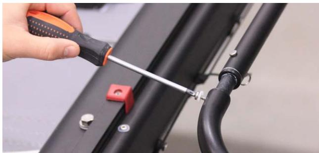
13. Fix the sliding bolt for the kick up tension. Push the bolt forward and fix the bolt while you're still pushing forward. The sliding bolt needs to be tightened firmly.
