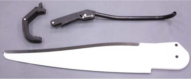
1. Assemble the upper and lower casting on the rudderblade. Use a flat screwdriver and grease.
