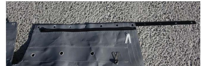
2. Insert the trampoline tie-rod into the slot on the rear of the trampoline.
