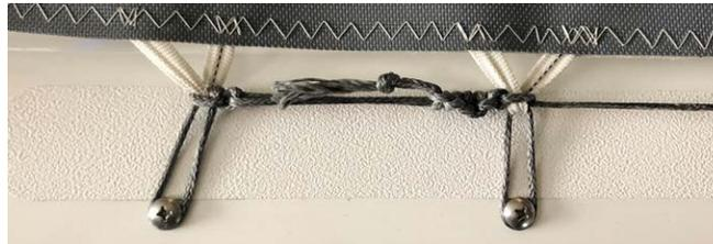
22. Finally tension the trampoline backwards from port to starboard.
