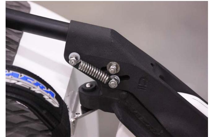
8. Take the philips screw out of the tillerarm.
