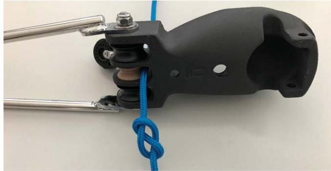
2. Feed the main halyard line through the sail groove towards the main halyard swivel hook. Feed it through both eyelets of the hook and guide the line around the mast sheeve.
