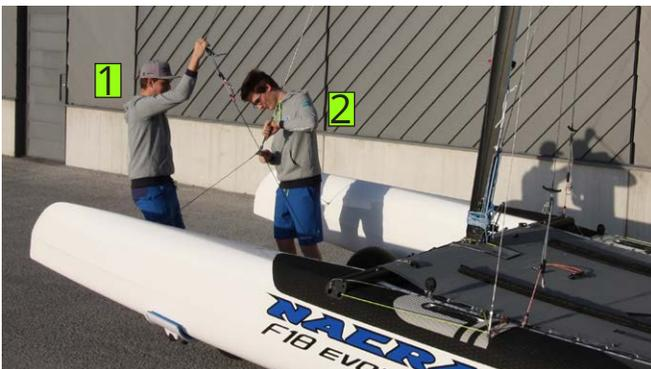
5. - **Person 1** Guides the mast by hanging easily on the trapeze lines.
