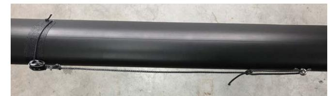
5. Install the 40mm carbo pivoting lead block. The cleat is facing downwards.
