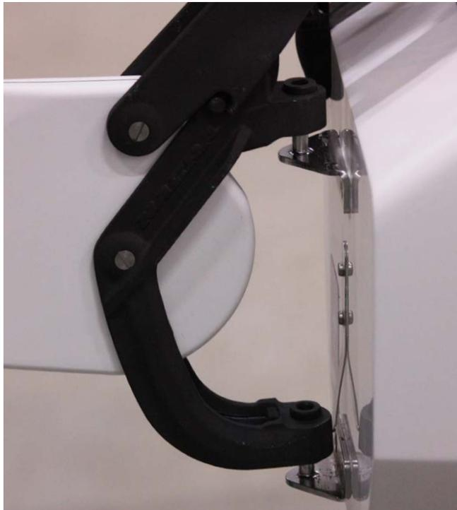
6. Push the casting all the way down and check if the retainer clip is over the casting.
