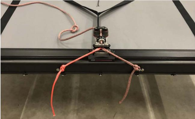
5. Move the traveler car to the side, a few centimeters away from the red traveler stop, and replace the knot from **step 1** towards the cleat on the traveler, making sure the car is not able to hit the (security) end stop.
