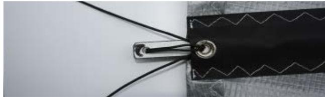
3. Push the batten forward for tension, tie the overhand knot at the same time. Just get rid of the wrinkles in the sail.
