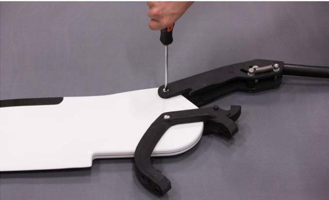
2. Use the self locking slot for the nylock nut at the port side of the casting.
