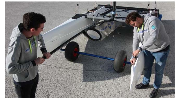
4. Knot the snufferline with a bowline around the pole and insert it in the slot of the ring.
