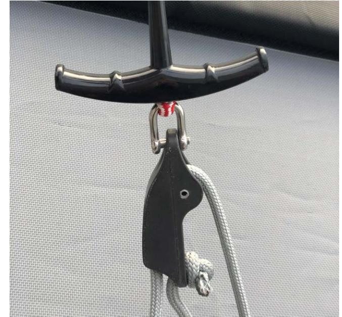
7. Knot the adjustable trapeze line to the trapeze shockcords.
