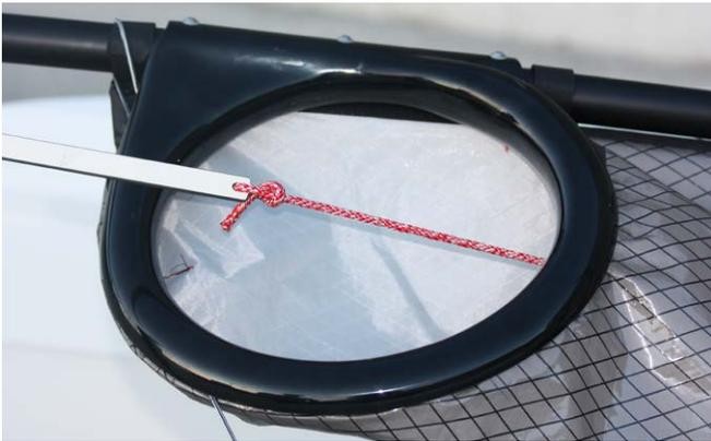
8. Attach the line temporary on the bridle wire.
