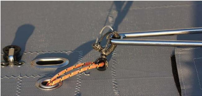
3. Feed the knot through the loop and pull.
