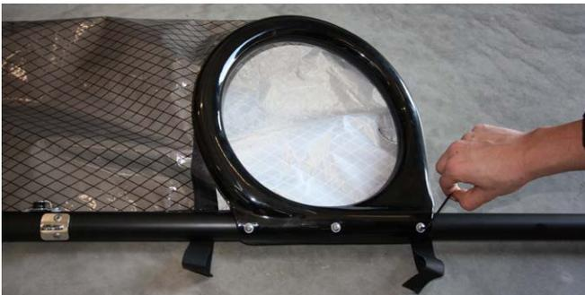
5. Install the snufferbag on the spipole using the velcro band.
