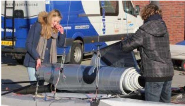
3. Guide the mainsail into the slot of the mast.
