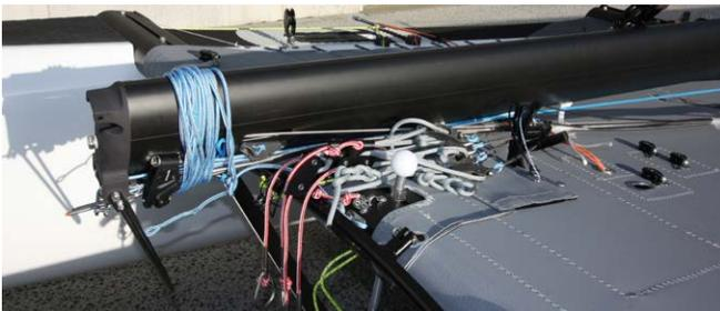
4. Check if the rigging and the shackles are connected on the mast as shown in **2.7 Fixing the stays**.
