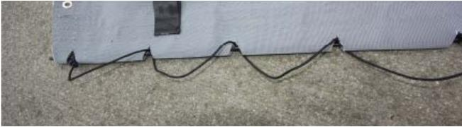
4. Fixate the trampoline with the trampoline plate on the buttons on the front crossbar. Make sure you bring the two loose flaps between the beam and the dolphin striker.
