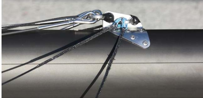
5. Attach the turnbuckle to the shroud eye and make sure you attach the ring from the continues mast rotation system on the inside of the turnbuckle.
