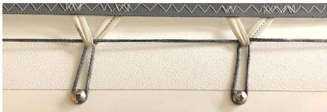
19. Now fully tension the trampoline sideways from front to rear.
