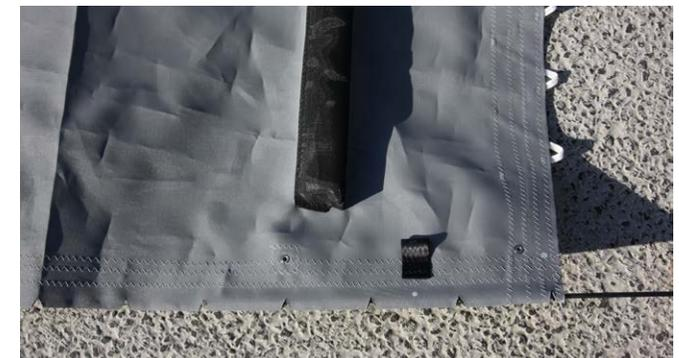
3. Loop the rear lacing line through the tie rod as shown in the picture. Start at the port side of the trampoline.
