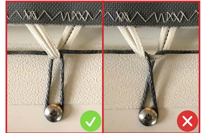
14. Tie the lacing line temporarily with half-hitch knot at the last loop.
