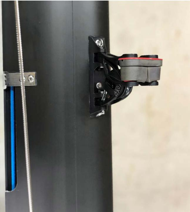
6. Feed the spinnaker halyard from inside to outside through the topblock.
