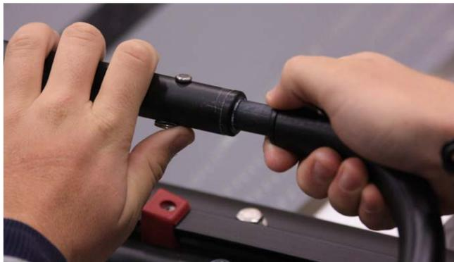
12. Check if the rod length is the same at both sides and pre-drill with the 3mm drill before you screw the philips screw.
