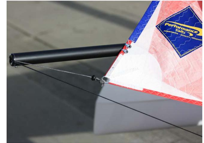
2. Un-knot the spinnaker halyard (temporarily fix on the 40mm cleat) and knot it to the head of the spinnaker with a bowline. Make sure the line is running free from all other rigging.
