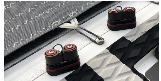
8. Attach the carbo 57mm ratchamatic single/swivel and the spring to the strap eye on both sides.
