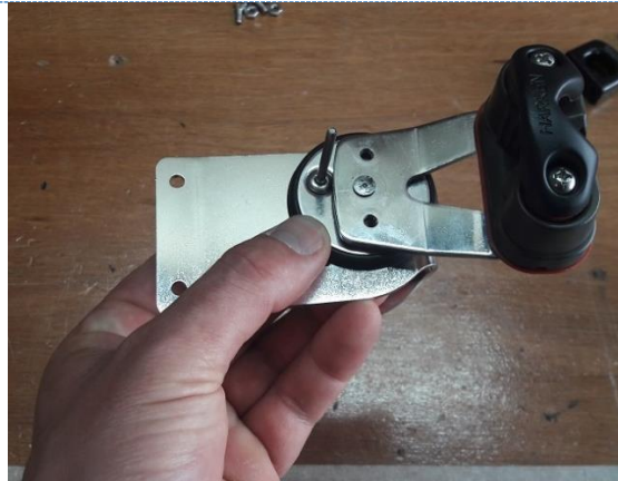
K. Mount the cleat on the received bracket. Use the 4.8x18 rivet
