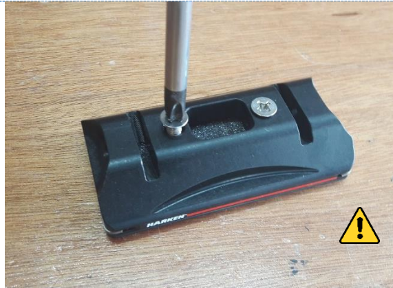
G. Screw the 2 screws back in the traveller car. The screws will hold the lock pin in place
