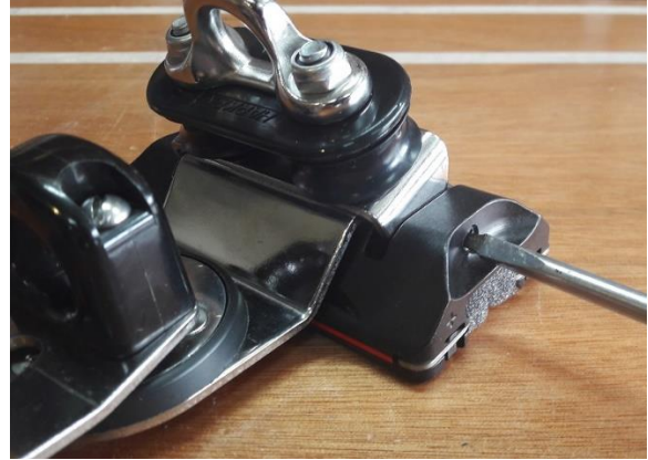
B. Use a small flat screwdriver to release the black stopper on the side. Be gentle, these are easy to ruin. When broken, use a drill 4mm and a needle to peel out the plastic
