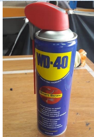
D. When the pin is salty and stuck, spray WD-40 en wait 5 minutes
