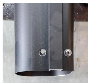
E. Dill a 5 mm hole in the insert. Use a 4.8x18 rivet
