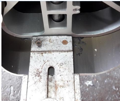
Measure if the insert sits straight in the beam.
