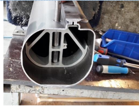
D. Slide the insert in the beam and place a pin or use a beambolt for positioning the insert.
