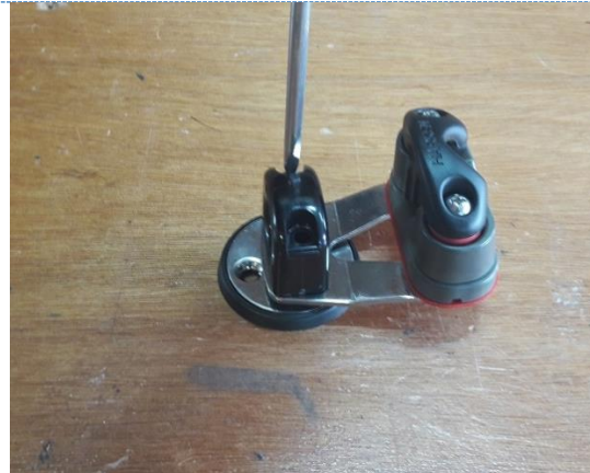
L. Screw the fairlead back in place on the cleat.
