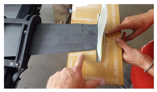
Note: The connection between the elevator and rudder is tapered. So when tighten the 2 supplied bolts the elevator connection will get solid.
