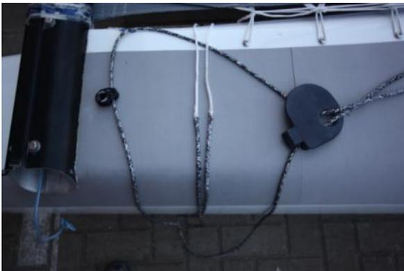
Lead the DBD rake trim line through the harken 29mm T2 single and splice both end into each other as illustrated in the pictures. After splicing sew the splice.
