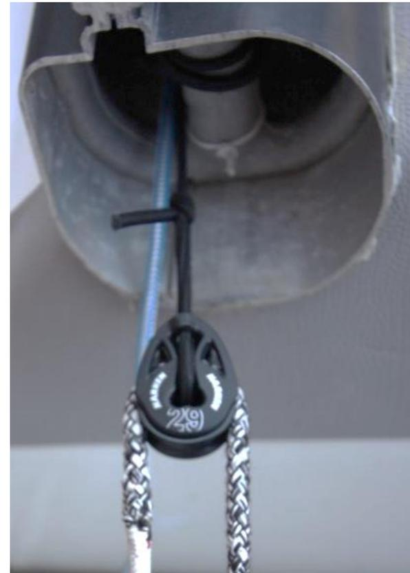
Tie the beam shockcord to the T2 single 29mm block.
