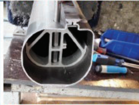
D. Slide the insert in the beam and place a pin or use a beambolt for positioning the insert.
