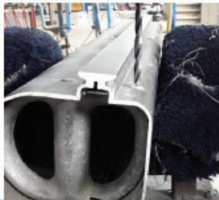
A. Drill out the rivet with a 5mm drill
