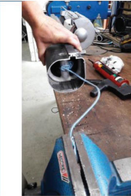
B. Tie a rope around the casting and pull firmly
