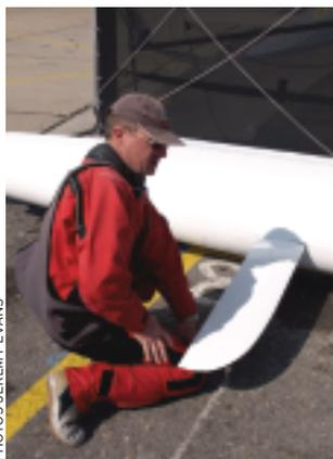
**Above** The Infusion's 'gybing' daggerboards have a thicker trailing edge at the top, allowing them to twist in their cases and provide extra lift upwind.
